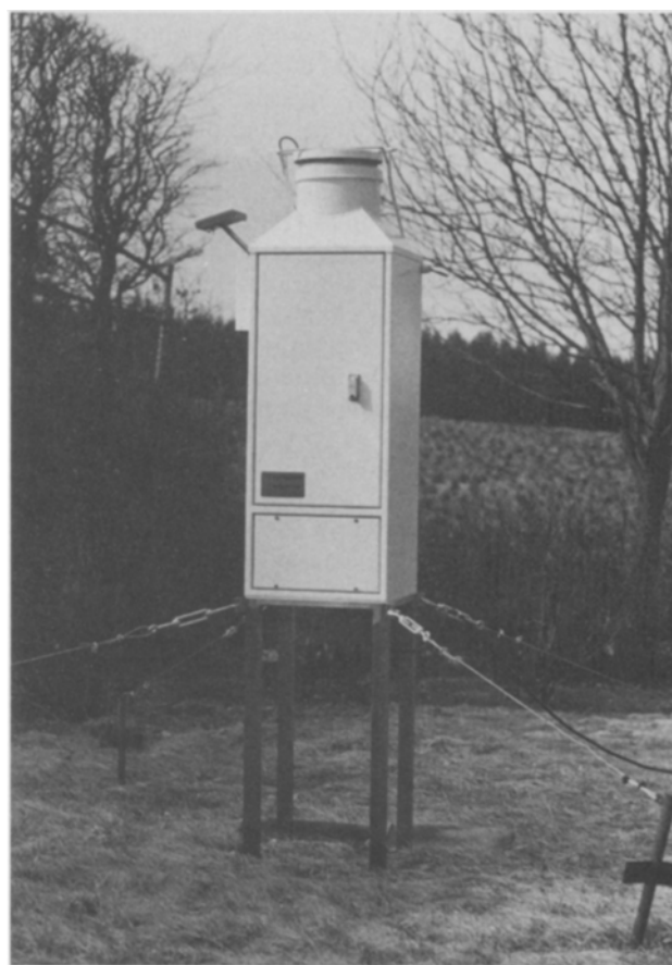
Figure 1. Automated precipitation sampler at field station.
